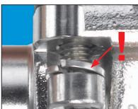
Insert the four bolts with their respective washers from the body side and tighten diagonally hand tight only. (Do not use force).
