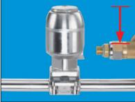
10. Move the actuated valve to the "closed" position. Move the manually operated valve to the "half open" position.
