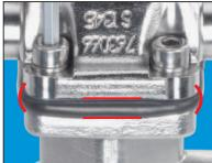
11. Tighten the connecting bolts diagonally in several steps with a suitable tool until the diaphragm is evenly compressed by 10 to 15% of its original thickness. If the diaphragm has an even outer bulge all round, correct compression has been achieved.
