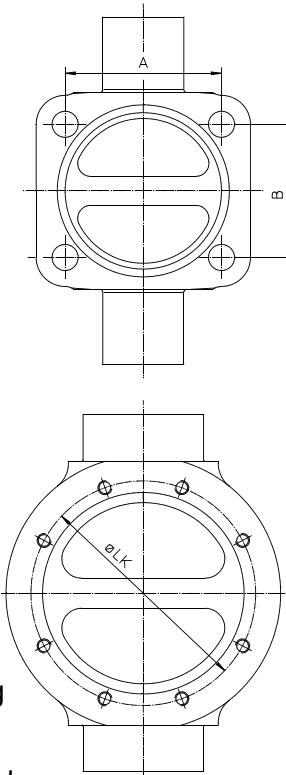
The guide values for torques given by GEMÜ are meant as an aid for determining the correct torque. They are only valid for undamaged bolts supplied by GEMÜ and for manual tightening by means of a torque wrench. Tightness and function is the most important criterion for each application. The bolts must be re-tightened, if necessary, depending on the application.
