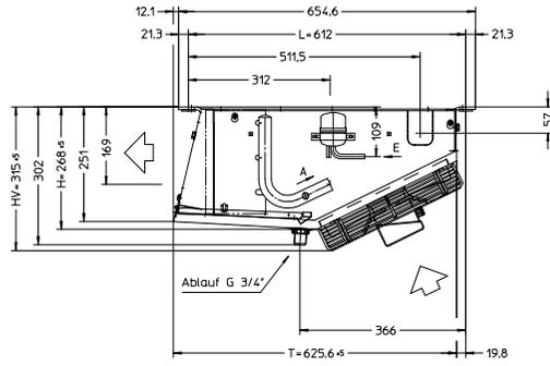
E (Inlet) -  $\varnothing 10 \times 1,0$  mm
