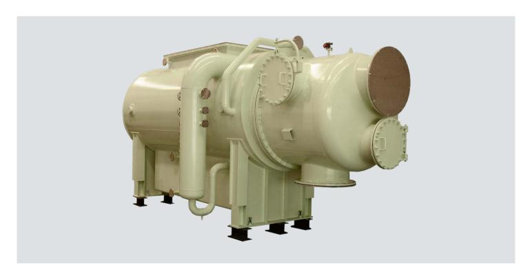
Surface condenser is the commonly used term for a water-cooled shell and tube heat exchanger installed on the exhaust steam side from a steam turbine in thermal power stations: coal fired power plants, oil fired power plants, CCGT, concentrating solar power (CSP), district heating, desalination plants, among others. Surface condensers are also used in applications and industries other than in power plants.
