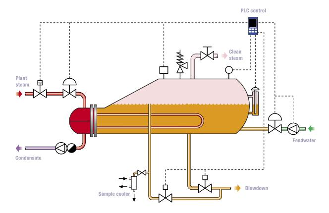
The treated feedwater is heated by a primary plant steam heating coil. This evaporates the feedwater producing secondary clean steam.
