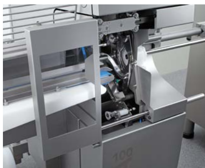
Shortest setup time due to comfort opening of front flap
