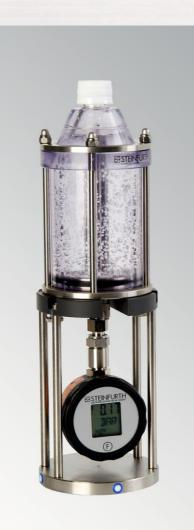
The Check Bottle TS 94.5 is used for monitoring the accuracy of the measuring heads of the  $CO_2$  tester TS 91.7. It consists chiefly of a polycarbonate container and an integrated digital precision instrument, combining manometer and thermometer.
