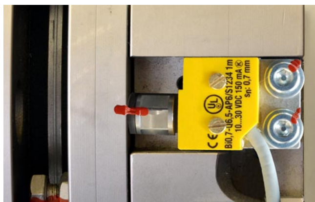
Contactless release monitoring with inductive proximity switches
